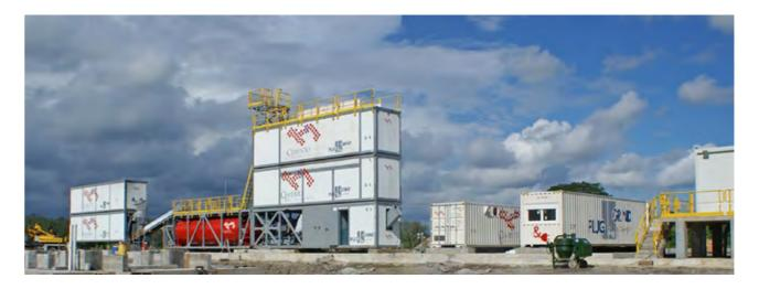
Plug&Grind® are installed. It should be pointed out that in this stage, the mill drive frequency drive is assembled together with the rest of the electrical works and the control room. The three local cabinets enable an easy and fast connection between containers. The "plug concept" is always borne in mind.
